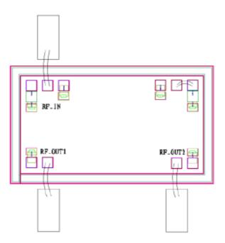
Note, customer can choose different coupling port, depending on different input and output direction, each coupling port has a 50  $\Omega$  load.
