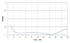
Switch OFF State Output Standing Wave Curve
